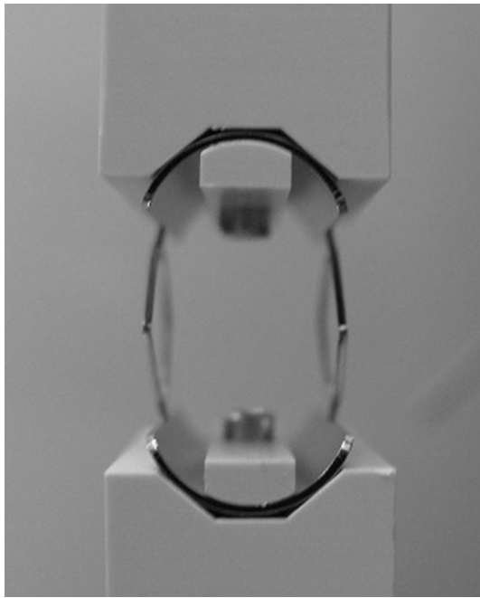
Fig. 3 Diamond-shaped specimen and tensile test setup
